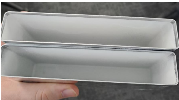
Application of ultra-pure aluminium hydroxides on li-ion battery cell casings using Alpha’s UltraCoat process
