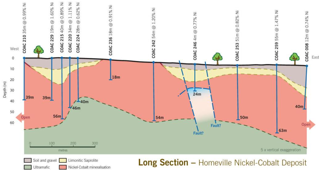
**Figure 2:** Long section of the Homeville Nickel-cobalt deposit showing location of the mineralisation to surface and drill holes.
