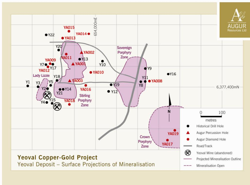
**Figure 2:** Plan view of the projected location of the mineralised bodies of the Yeoval Copper-Gold-Molybdenum-Silver deposit, at Yeoval, central New South Wales, Australia.
