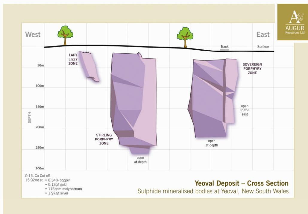
**Figure 1:** 3D modelled cross section of the Yeoval Copper-Gold-Molybdenum-Silver deposit, at Yeoval, central New South Wales, Australia.
