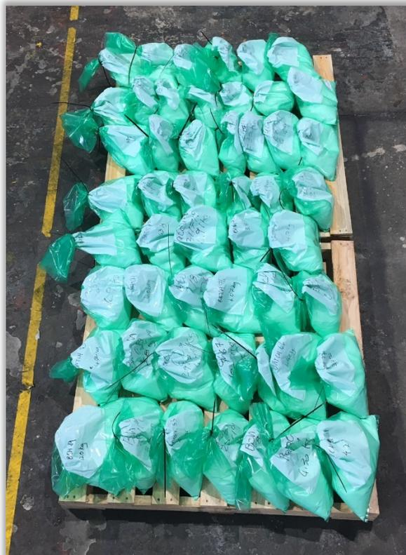
2 x pallets, totalling 212kg of high-purity Al crystal produced in Pilot campaign 2A
