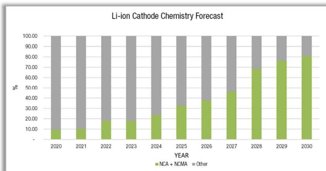
Aluminium bearing cathode active chemistries (NCA + NCMA) are forecast to represent 80% of all lithium-ion battery cathode chemistries by 2030
