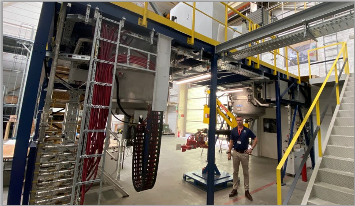
Synthetic sapphire growth units operating at Ebner-Fametec, Austria. These units are identical to those under construction for Alpha Sapphire and are currently being used to qualify Alpha's HPA feedstock.
