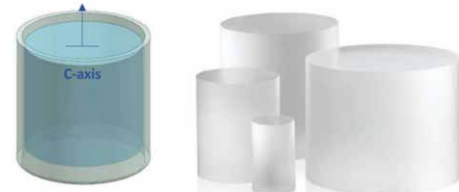
C-axis ingots produced from an c-axis grown McSAP sapphire boule showing high utilisation
