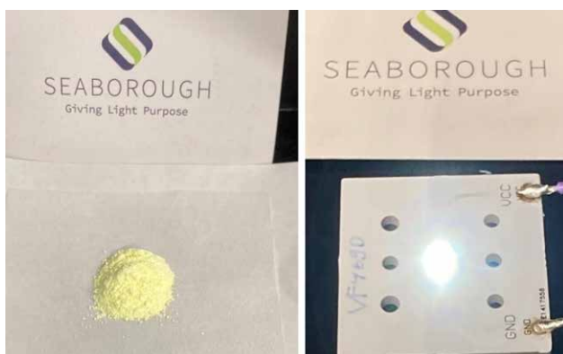
YAG:Ce nano-phosphors made with Alpha's 5N Al-Nitrate (left photo). The same phosphors emitting on top of a mid-power LED chip, showing close to 100% quantum yield (right photo)
