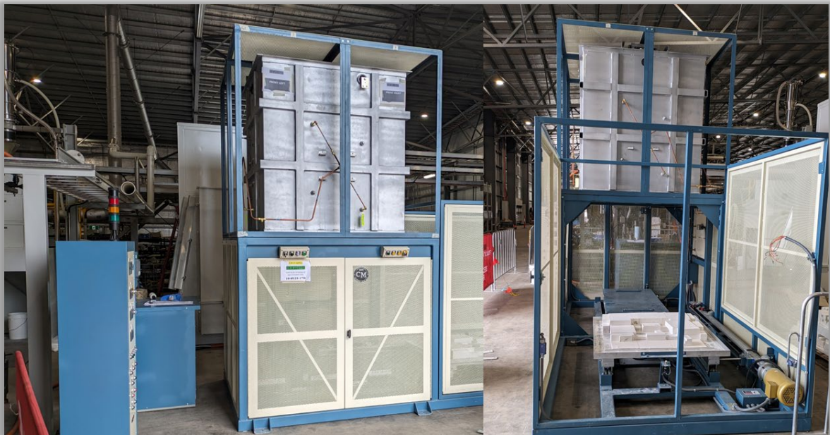
Sinter oven for HPA tablets – delivered to site
