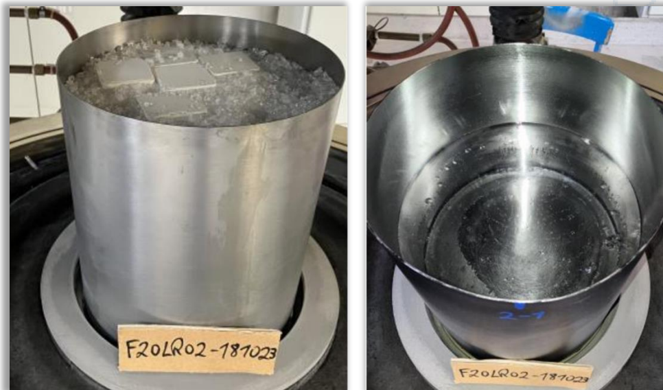
Pre-melt crucible packed with Alpha HPA tablets (LHS). Completed, single crystal sapphire boule (RHS). (scale approx. 20cm diameter)
