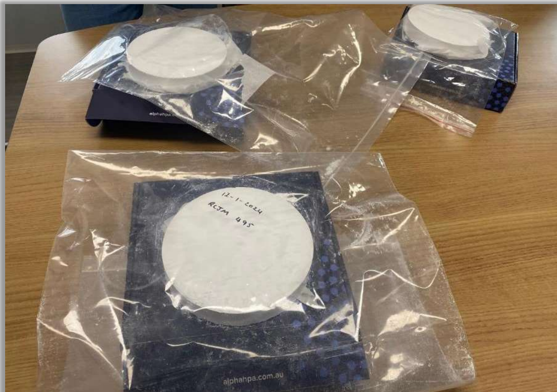
Sintered high-density circular HPA tablets – custom designed for the Ebner-Fametec growth units
