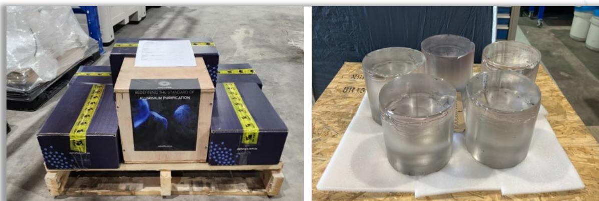
5x 30kg boules of good body sapphire (RHS) and first sapphire boule packaged and sent to customers for qualification testing (LHS), together with a 100kg HPA tablet sale
