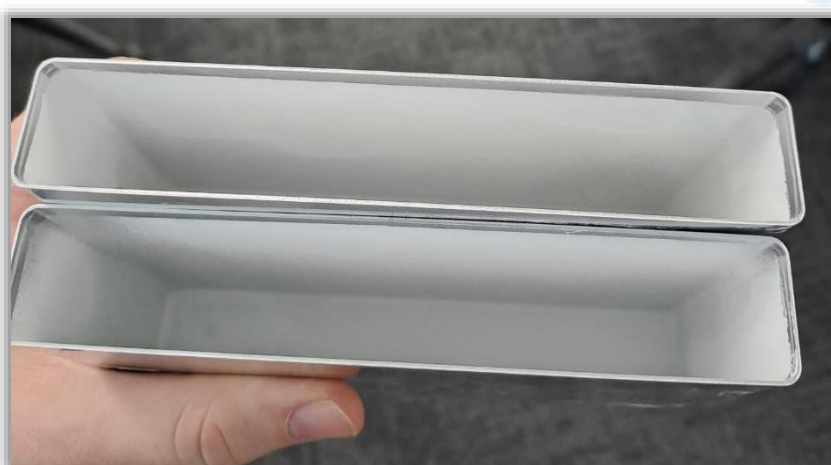
Application of ultra pure aluminium-hydroxides on li-ion battery cell casings using Alpha's UltraCoat process
