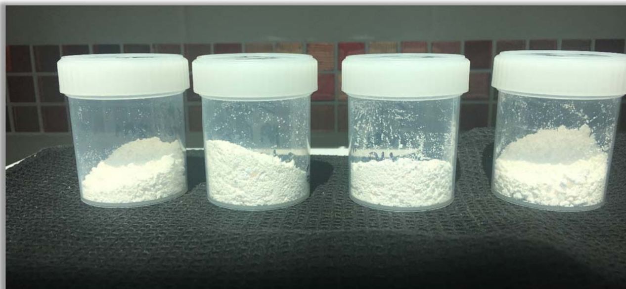
Figure 1: High Purity Alumina produced from the second SX mini-rig run
