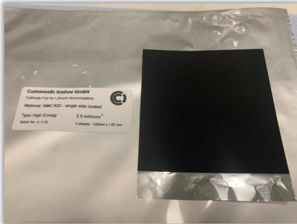
NMC622 cathode foil impregnated with Alpha HPA
