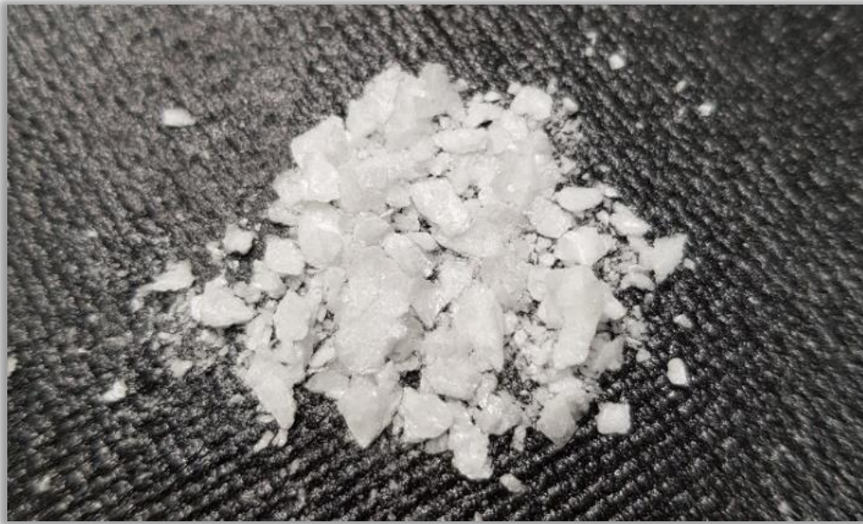
High-purity (99.995%), lithium-ion cathode pre-cursor
