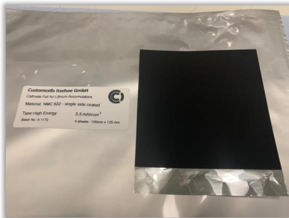
NMC622 cathode foil impregnated with Alpha's high purity alumina
