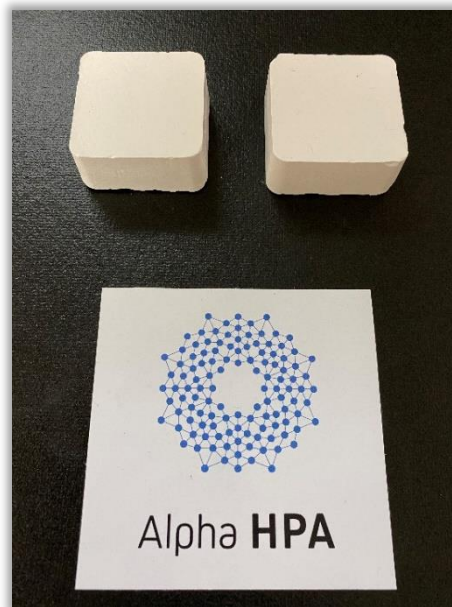
HPA pellets for sapphire glass end-users (~45 x 45 x 20mm)
