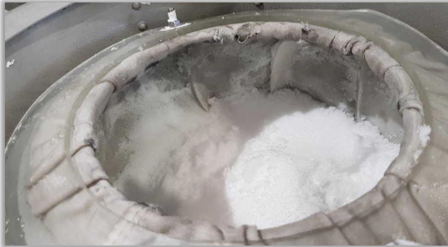
A centrifuge batch of high-purity pre-cursor product (approx. 2kg) produced at Alpha's demonstration facility
