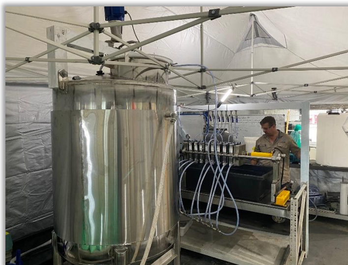
Demonstration scale pre-cursor circuit generated 99.998% purity HPA
