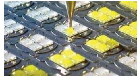
Addition of YAG phosphors to LED lighting circuits
