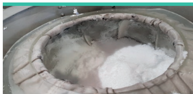
A centrifuge batch of 5N purity aluminium nitrate-nonahydrate product produced at Alpha's demonstration scale facility
