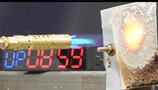
ULTRA-COATED ALUMINIUM Layer integrity intact after 9 minutes under butane flame
