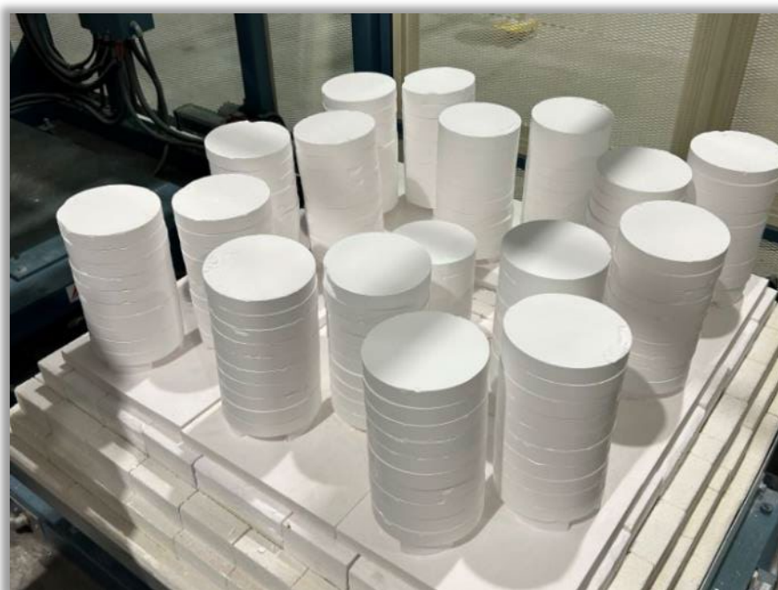
A production batch of densified, sintered HPA disc tablets (each tablet ~850g with density of >3.5g/cm 3 )
