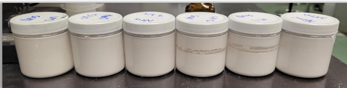
Alpha's samples of Ultra fine nano-alumina ( \sim 100 nm) dispersions – prior to customer despatch
